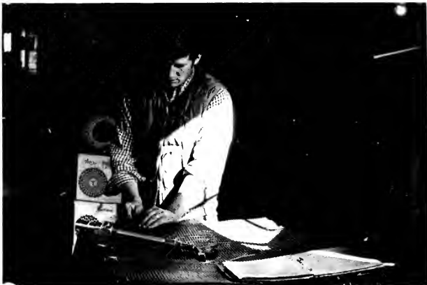
Will replaces screening on suction cages.
